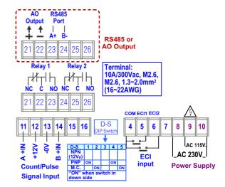
Please check the voltage of power supplied first, and then connect to the specified terminals. It is recommended that power supplied to the meter be protected by a fuse or circuit breaker
