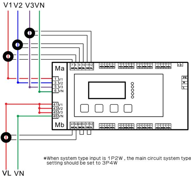
\*When system type input is 1P2W, the main circuit system type setting should be set to 3P4W
