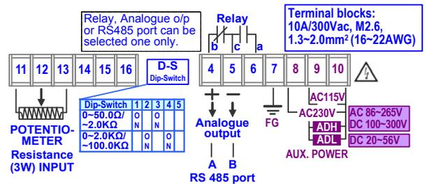
Please check the voltage of power supplied first, and then connect to the specified terminals. It is recommended that power supplied to the meter be protected by a fuse or circuit breaker.
