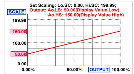
The range between RoHS and RoLS should be over 20% of span at least; otherwise, it will be got less resolution of analogue output.
